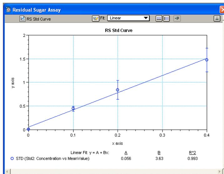
**RS assay standard curve.** A standard curve plotted and used for deriving the concentration of residual sugar in wine samples.
