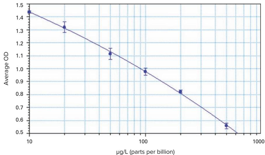
**Melamine assay sensitivity.** Melamine standard curve demonstrating assay sensitivity down to 10 ppb.
