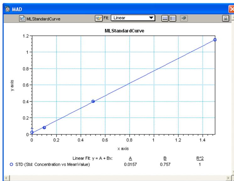
**MAD assay standard curve.** A standard curve was plotted with linear curve fit and used to derive the concentration of malic acid in wine samples.
