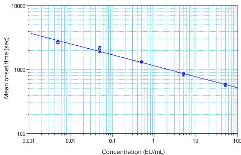
**Pyrochrome assay standard curve.** Pyrochrome Assay log-log standard curve generated in SoftMax Pro GxP Software version 5.3. Standard curve was composed of five dilutions of control standard endotoxin in triplicate.
